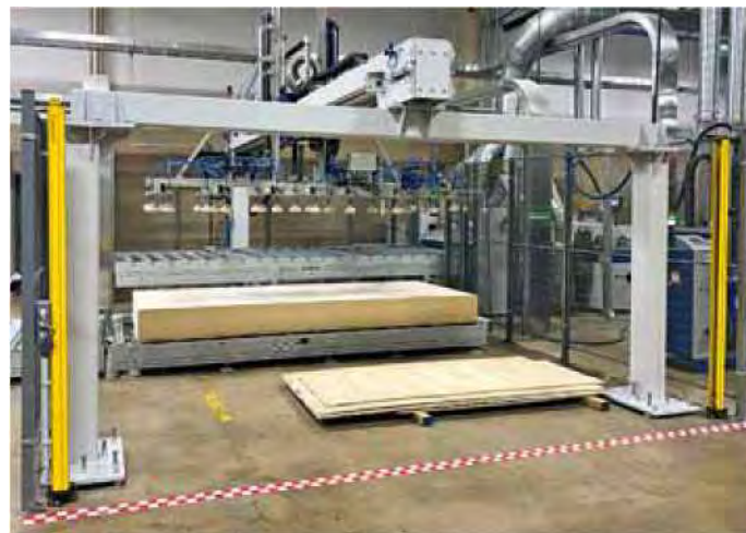
Installed gantry feeder with protection board storage. Positioned in front of a panel cleaning and coating system at a renowned panel finishing company. Version as seen in the CAD drawings (1 to 3)
